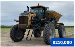
**2018 AGCO Rogator RG1300C,** 1780 hours, AGCO turbo diesel engine, 4-speed hydrostatic auto. trans., AGCO adjustable axles, 4WS, New Leader 304 SS 11T L4258G4 spreader body with MultApplier, Raven Viper 4, RGL 600 lightbar, A/C, AM/FM radio, air ride seat, Agri-Cover electric roll tarp, rear camera, fenders, 380/90R46 row crop tires.
