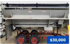
**2017 GVM 11.0T Double Duty FR Spreader,** painted 409 SS with 304 SS cross members and mounts, 13 ft  $\times$  102 in. wide, 330 ft<sup>3</sup> capacity, rear camera, 3-ton 95 ft<sup>3</sup> 5 ft  $\times$  102 In. wide capacity Fusion Insert, bin level sensor, Raven CAN Nodes, Fusion Cable-Lok roll tarp with SS bows.
