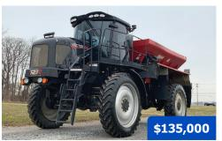
**2017 RBR Vector 300**, 2958 hours, Cummins QSB 8.3 300 hp diesel engine, Allison 6-speed auto. trans., New Leader L4000G4 spreader body, Viper Pro, A/C, air ride seat, 380/90R46 tires (50% remains). Also includes (4)Firestone 650/65R38 floater tires. SN: M1700598 (PA) **No. U1422**
