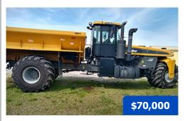
**2015 AGCO TG7300 TerraGator**, 2100 hours, AGCO 330 hp diesel engine, CVT auto. trans., painted 409 SS New Leader L4000G4 14 ft spreader, Viper Pro, AgCommand controller, Slingshot ready, A/C, premium leather air ride seat, 1000/50R25NHS front tire, 1000/50R25 rear tires (70% remains). Engine rebuilt 6/18 by AGCO under warranty, has 500 hours on it.
