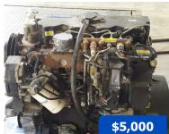
2010 4660 SpraCoupe Perkins Diesel Engine 1104D, 874 hours, 4 cylinder, 4.4L (269 in.3), 125 hp (93 kW) at 2200 rpm. Engine includes: alternator, starter injection pump, turbo charger, and primary fuel filter and housing. (PA)
